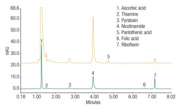
Figure 4. Separation of WSV in tablet. Orange trace: 210 nm; blue trace: 270 nm.
