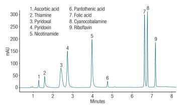
Figure 2. Separation of a water-soluble vitamins standard on an Acclaim PA2 column (150  $\times$  2.1 mm, 2.2  $\mu m$ ) recorded at 210 nm.
