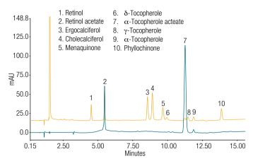
Figure 5. Comparison of the standard mixture (orange) with  $100 \mu$ g/mL and the vitamin tablet (blue) at a wavelength of 280 nm.
