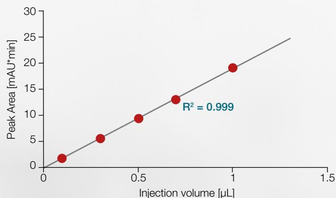
Autosampler linearity for even low injection volumes, here from 100 nL to 1 µL.
