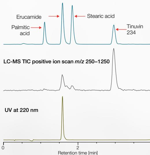
Unlike mass spectrometry and UV, the CAD is able to measure all analytes in the sample. Mass spectrometry (MS) requires the analyte to form gas phase ions while response by a UV detector depends upon the nature of the chromophore.
