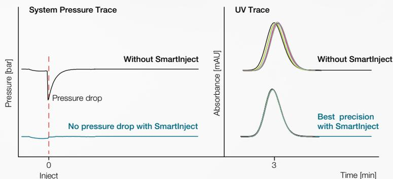
Significant reduction of pressure drop after injection using SmartInject Technology resulting in improved retention time reproducibility (6 replicates) and enhanced column lifetime.
