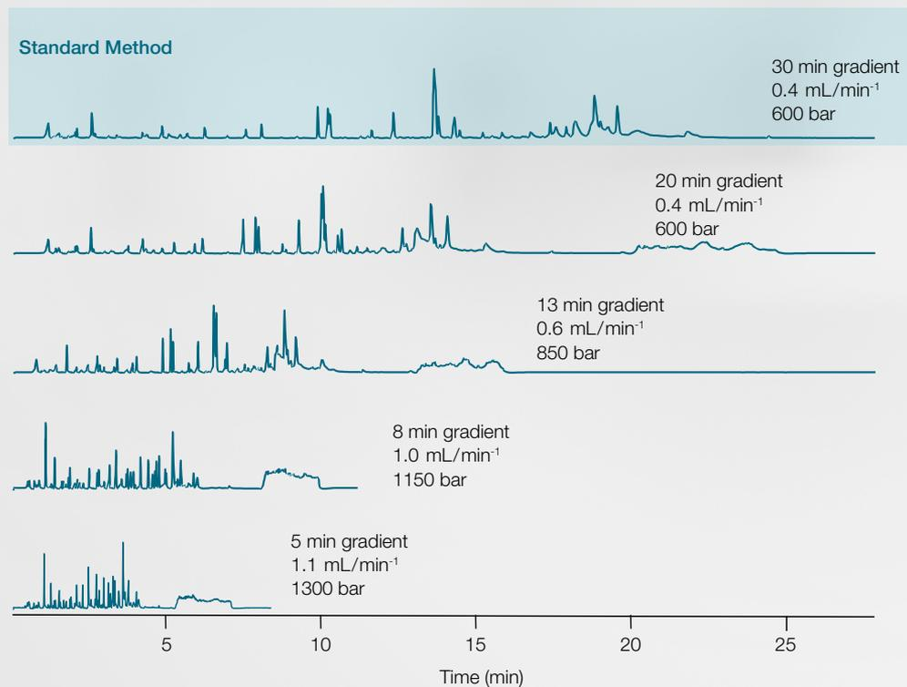
**Accelerated peptide mapping utilizing the full power range of the Vanquish Horizon UHPLC system while maintaining 100% sequence coverage using a Thermo Scientific™ Acclaim™ RSLC 120, C18, 2.2  $\mu\text{m}$  column.**
